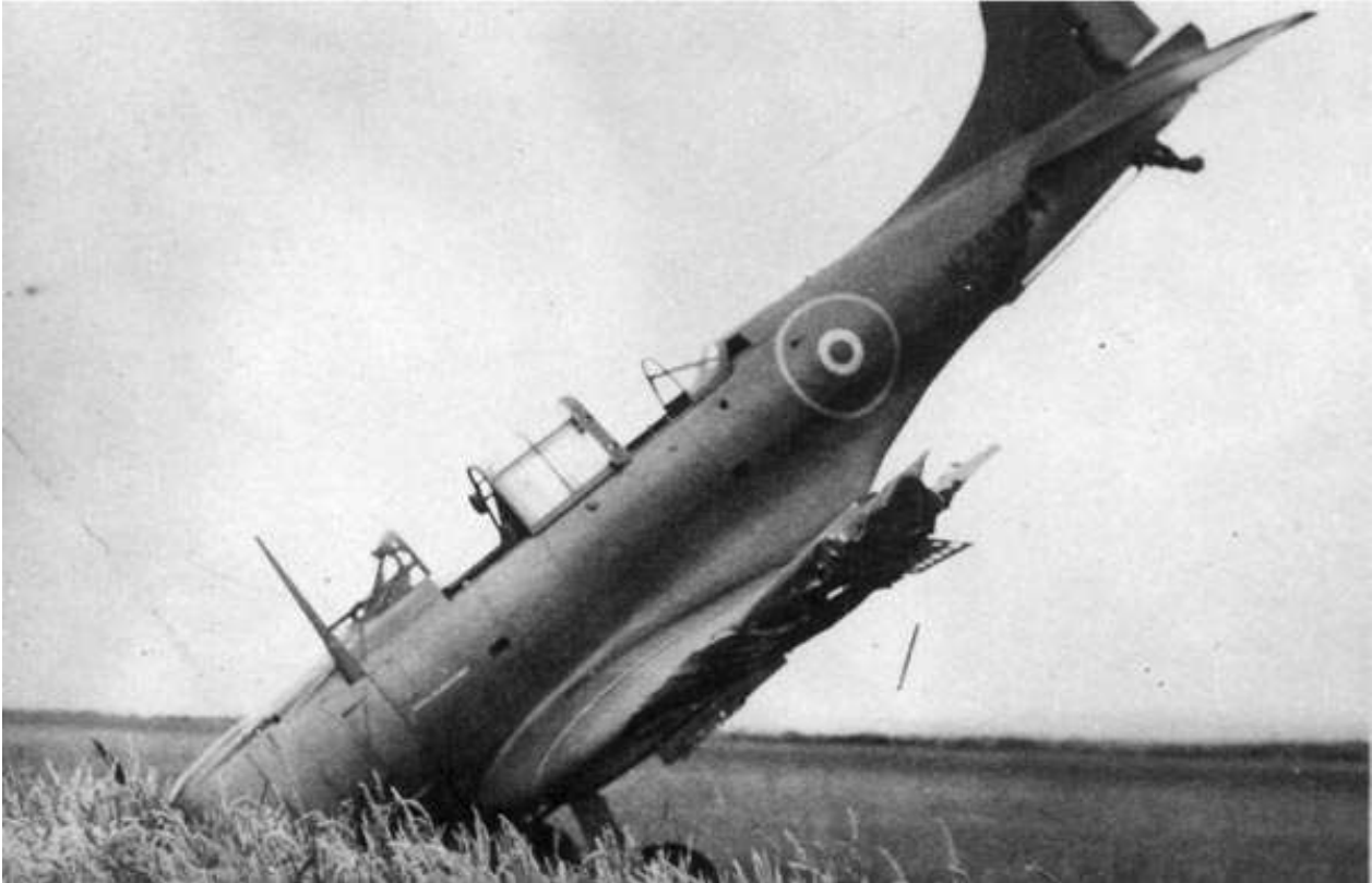
Dauntless "nose over" taxiing accident. Seagrove, 1943. Image courtesy of the Air Force Museum of New Zealand
